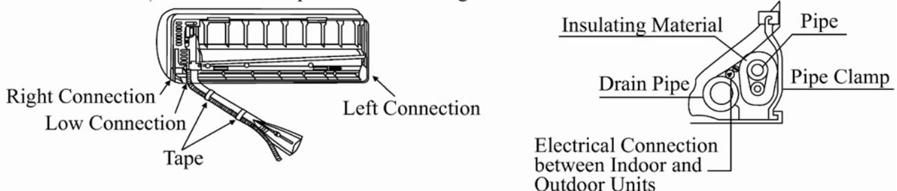
Installation of the Connection Pipe Clips (Left or Left-Back Connection):
