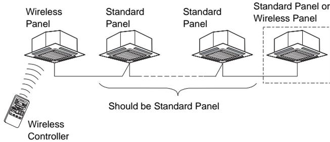
In case of applying two (2) air panels for wireless control, the setting of main and sub receiver part is required. Refer to the item 4.4.5 "Optional Function Setting" for the dip switch setting procedures.
