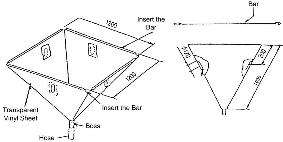
Inner Side of Ø120 hole should be covered with felt sheet to insert the spray nozzle.
