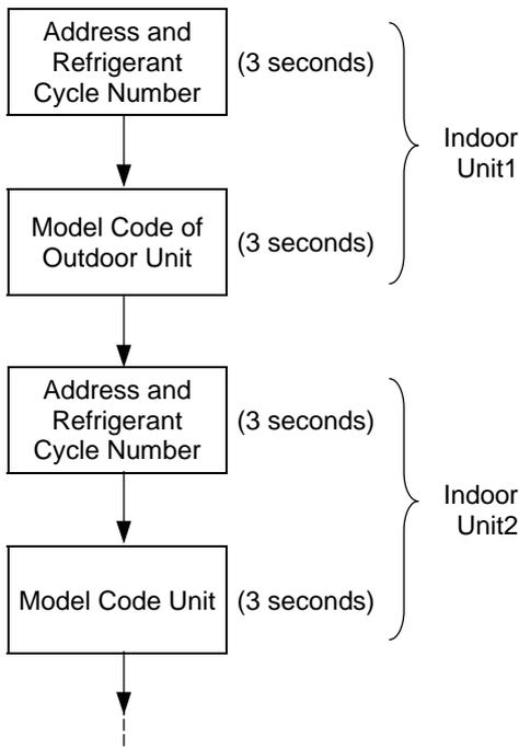
The indication of the above items ❶~❷ for all the indoor units connected the remote control switch is completed, the remote control switch is returned to the normal condition.
