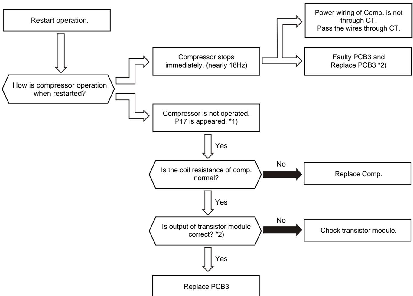
\*1): P17 is shown at 7-segment on the outdoor unit PCB.
