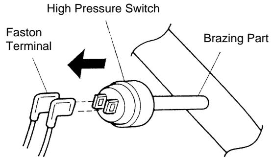
**A-2. Removing High Pressure Switch**
