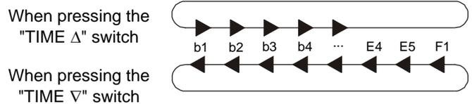
c. Press the "CHECK" switch, and the setting condition of the optional function is changed as shown below.
