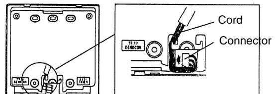
3. Disassemble the panel by removing two screws.
