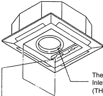
Thermistor for Air Outlet Temperature (THM2)
