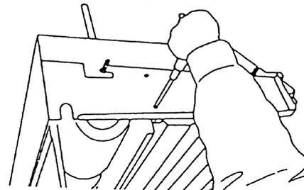
8. Attach the drain pan and lower cover according to the reverse procedures in the item, (4).
