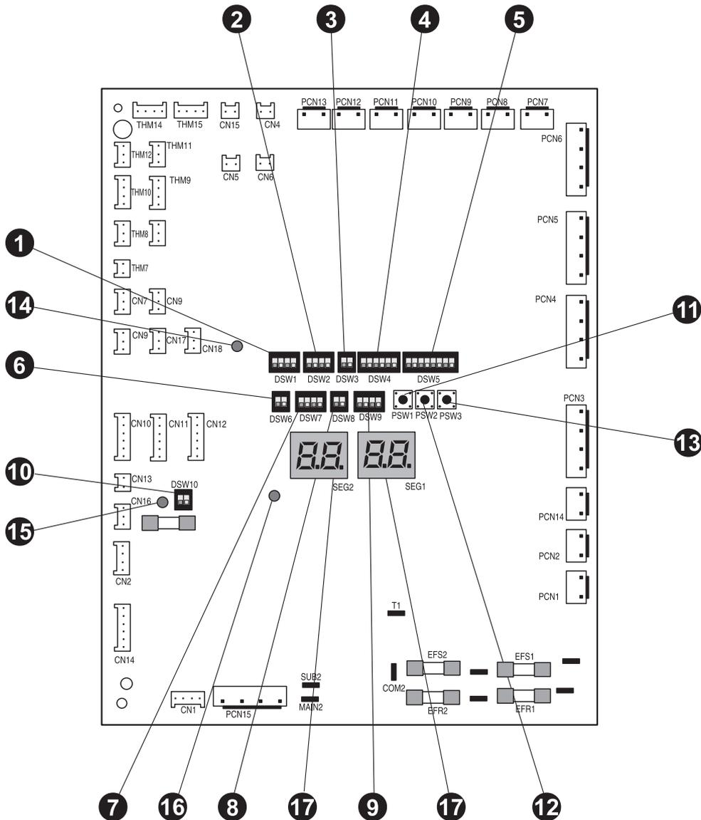
■ Dip Switches and LED Functions on Outdoor Unit Printed Circuit Boards
