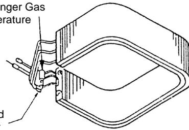
Thermistor for Indoor Heat Exchanger Liquid Pipe Temperature (for Freeze Protection) (THM3)
