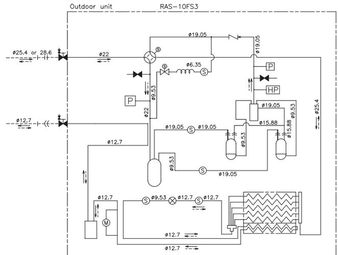
Fig. 3.2 Refrigeration Cycle of Outdoor unit (RAS-10FS3)
