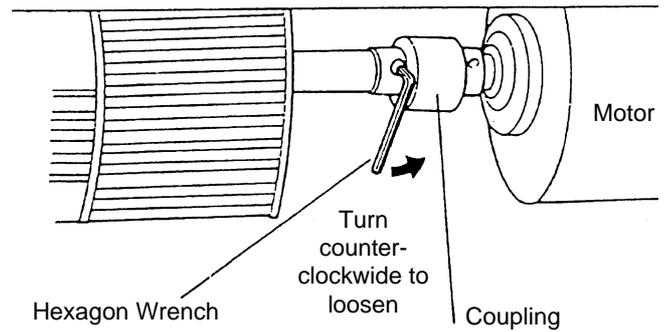
6. Remove the motor, after removing the fixing band for the motor. Perform this work by supporting the motor by hand.
