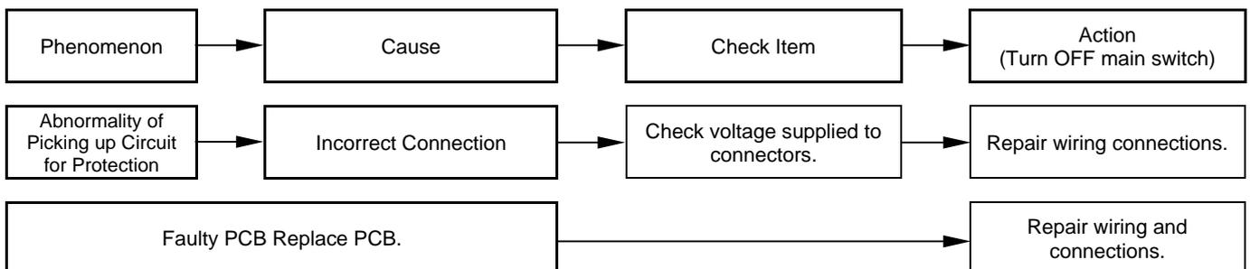
\*1): Check wiring system connecting to PCN14 and PCN2 on PCB1.
