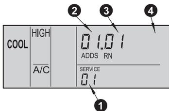
b. At the condition of the above item (a), press the "TEMP ∇" switch or the "TEMP Δ" switch of the remote control switch and the indoor unit for which the optional function is to be set, can be changed.
