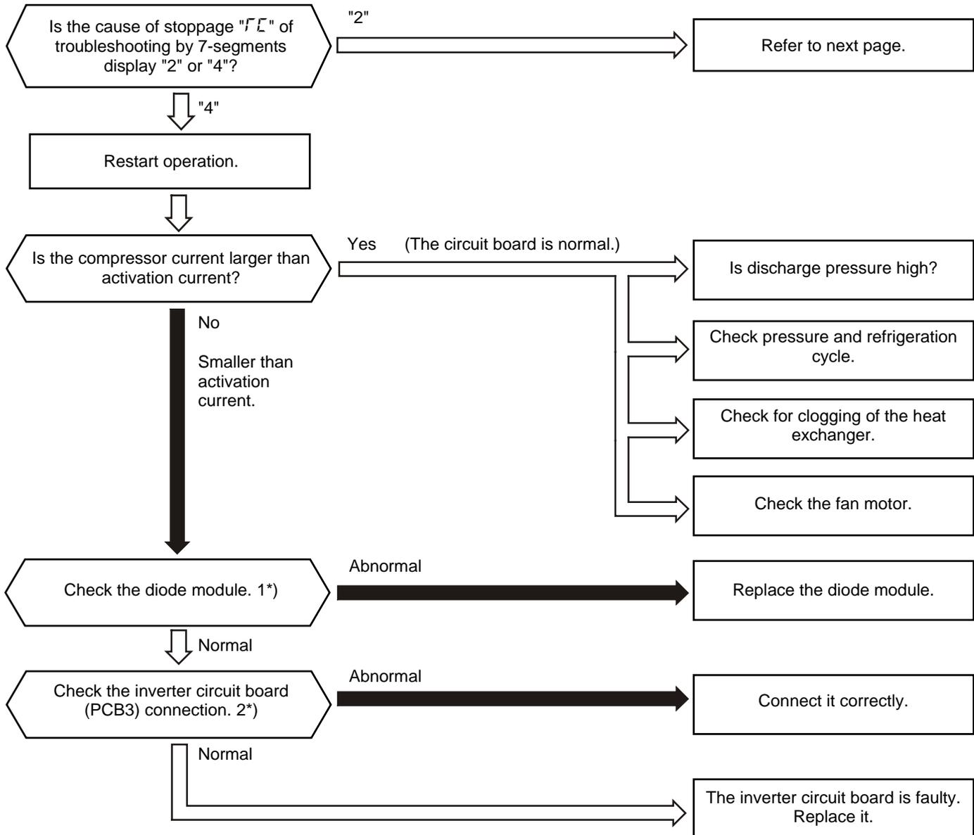
\*1): Regarding the checking method for diode module, refer to page 1-92.
