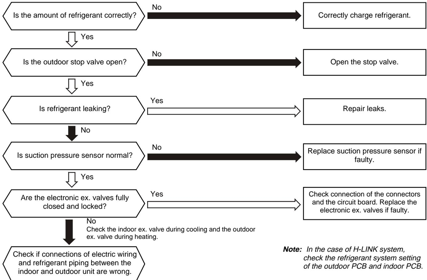
**Note:** In the case of H-LINK system, check the refrigerant system setting of the outdoor PCB and indoor PCB.
