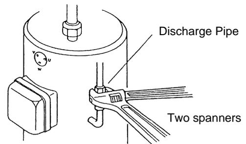
8. Disconnect the suction pipe of the compressor. Use two spanners when disassembling the flare-nuts.
