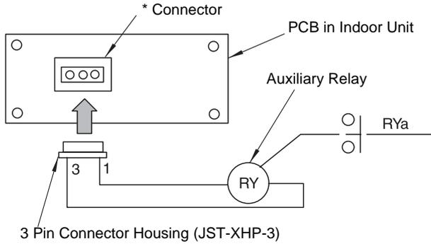
■ Picking Up "Thermo-ON" Signal during Cooling Operation (Only for RCD-FSG(E) and RPF(I)-FSG(E) models)
