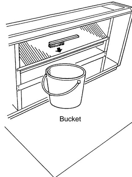
6. Spray cleaning water over the fins of the heat exchanger.
