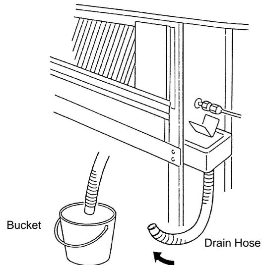
5. Removing Dust on Heat Exchanger
