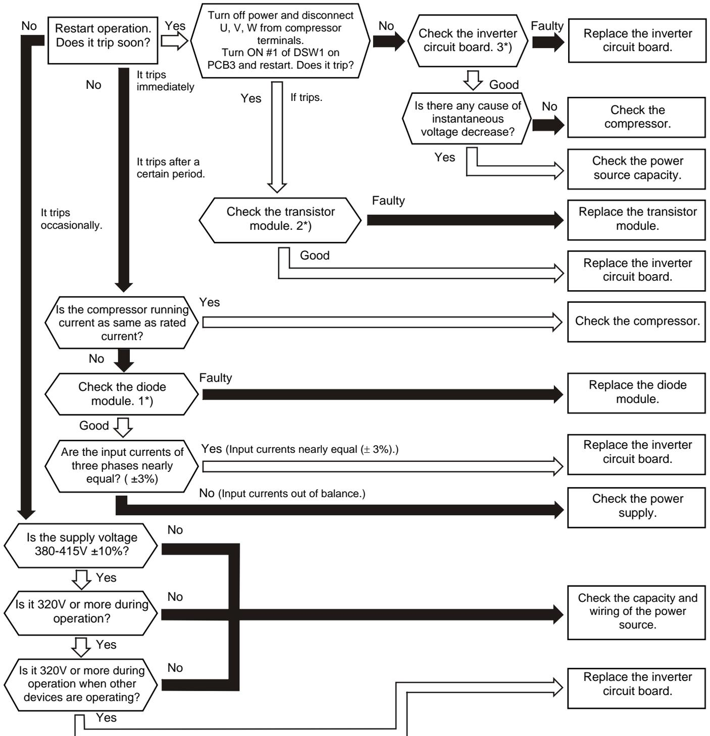
1\*): Regarding or replacing the checking method for the diode module, refer to page 1-92.
