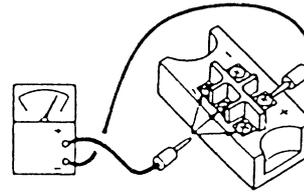
c. By touching the - side of the tester to the - terminal of the diode module and the + side of tester to the ~ terminals (3 Nos.) of the diode module, measure the resistance. If all the resistances are from 5 to 50 k $\Omega$ , it is normal.
