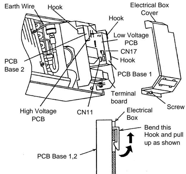
6. After the completion of replacement of PCB, connect the connectors to the PCB in the reverse procedures of removing. And firstly set the high voltage PCB to the electrical box and then set the low voltage PCB to the electrical box.
