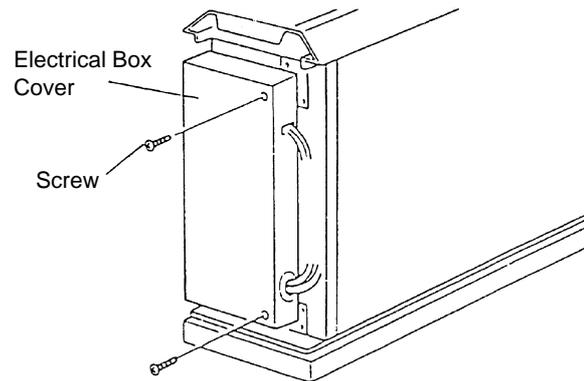
6. The electrical box can be turned up to an angle of 90° by removing two (2) fixing screws and unhooking the hook at the rear side of the electrical box.
