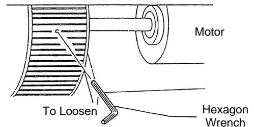
8. Remove the fan motor by sliding it backwards after removing the fixing plate. Pay attention not to drop it.
