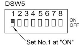
No. 1 of DSW5 is set at OFF before shipment. Turn OFF the main switch and set the dip switch.
