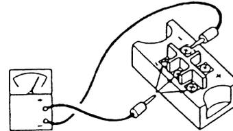
d. By touching the + side of the tester to the - terminal of the diode module and the - side of tester to the ~ terminals (3 Nos.) of the diode module, measure the resistance. If all the resistances are greater than 500 k $\Omega$ , it is normal.
