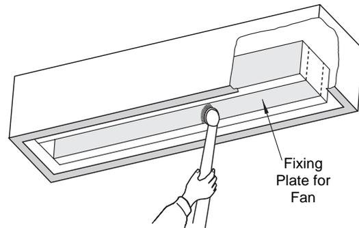
4. Removing Dust on Heat Exchanger
