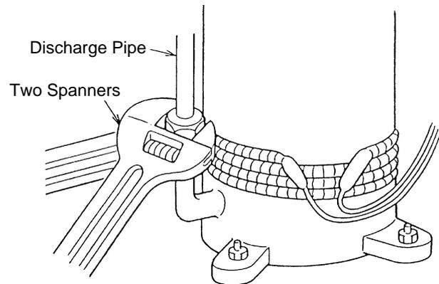
8. Remove the flare-nut at the compressor side, and disconnect the oil piping. There is a possibility that the oil may flow from the inside of the oil pipe. Therefore, prepare an oil pan, etc. to collect the oil.
