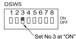
No. 3 of DSW5 is set at OFF before shipment. Turn OFF the main switch and set the dip switch.
