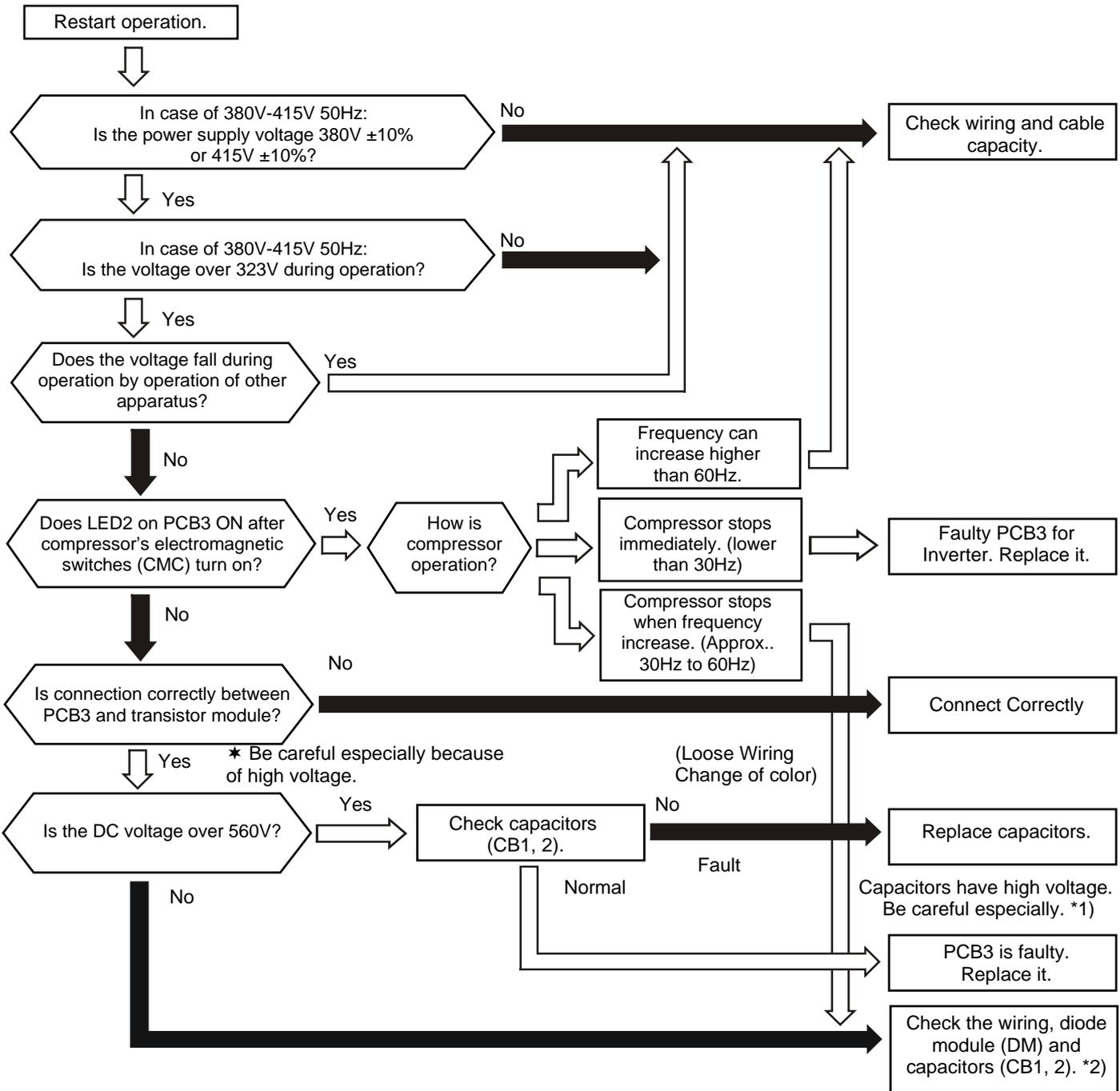
\*1): If capacitor has high voltage, perform the high voltage discharge work refer to item 1.3.6.
