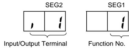
This display indicates that the function No. 1 (Fixed Heating Mode) is set at input 1.
