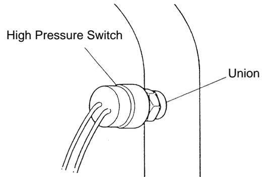
**B. Removing High Pressure Sensor and Low Pressure Sensor**
