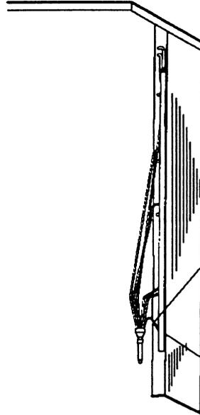
Thermistor for Evaporating temperature (THM10 and THM11)
