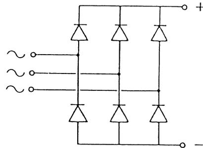
If items (a) to (d) are performed and the results are satisfactory, the diode module is normal. Measure it under 1 k $\Omega$  range of a tester. Do not use a digital tester.
