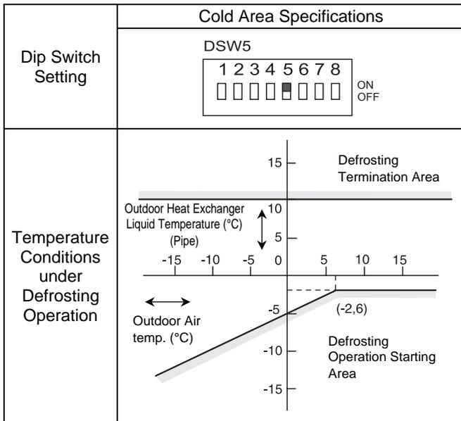
No. 5 of DSW5 is set at OFF before shipment. Turn OFF the main switch and set the dip switch.
