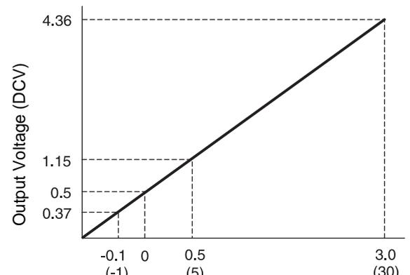
Output Characteristics of Low Pressure Sensor
