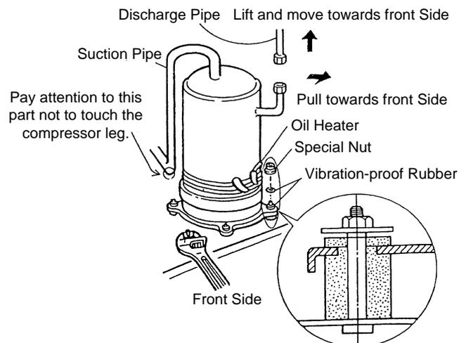
Pull out the compressor toward the front side, and remove the vibration absorbing rubbers.
