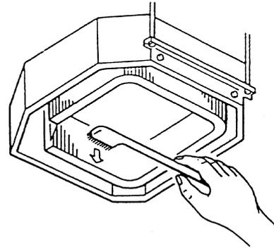
3. Suspend the cleaning water collector from the indoor unit.
