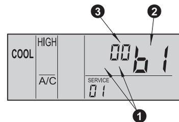
b. Press the "TIME ∇" switch or the "TIME Δ" switch, the optional function item is changed as shown below.
