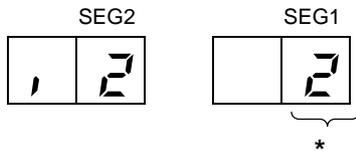
\*) This number is increased by 1 by pushing PSW2 while PSW1 is being pushed. This number is decreased by 1 by pushing PSW3 while PSW1 is being pushed.
