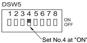
No. 4 of DSW5 is set at OFF before shipment. Turn OFF the main switch and set the dip switch.
