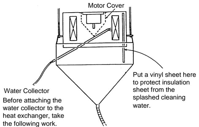
5. Put a vinyl sheet around the heat exchanger so that cleaning water will not be splashed over the insulation surface and drain-up pump. Fix the vinyl sheet on the side plate of the heat exchanger by using tape with adhesive. Seal the gap between vinyl sheets using tape with adhesive.
