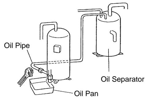
9. Remove the suction pipe of the compressor.
