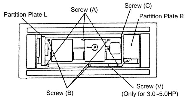
4. Remove the casing by pushing four (4) extruded parts at the lower part of the casing, which consists of two parts.
