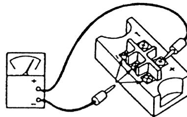
b. By touching the - side of the tester to the + terminal of the diode module and the + side of tester to the ~ terminals (3 Nos.) of the diode module, measure the resistance. If all the resistances are greater than 500 k $\Omega$ , it is normal.
