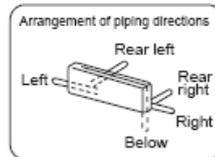
Note: Cooling only units don't have Drain-elbow
