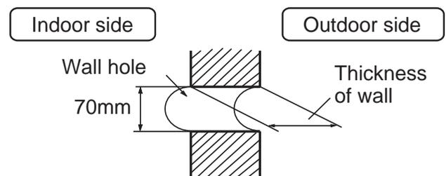
(Section of wall hole) Ⓒ Piping hole pipe
