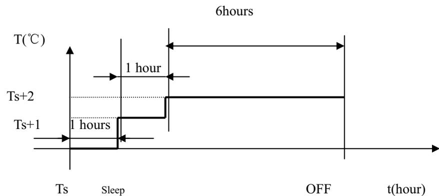
As shown in the above diagram, after running for 1 hour under refrigerating mode and dehumidification mode, the setting temperature will increase  $1^\circ\text{C}$ ; after another 1 hour, it will increase  $1^\circ\text{C}$  again, and after 6 hours, it will cease;
