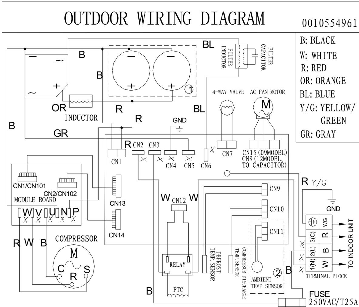
CAUTION: The ① can be capacitor board or the capacitor with a clip, which are optional for different unit. The ② are optional for different unit. In the module board, the "CN1, CN2" is for "9000BTU" units; The "CN101, CN102" is for "12000BTU" units.
