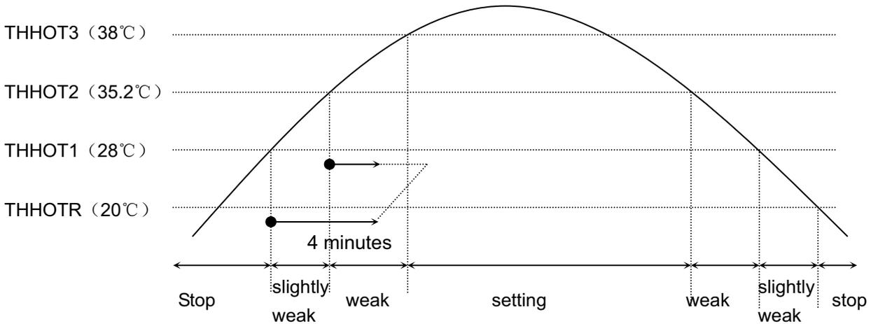
To control the indoor fan motor as shown in the table above according to the heat exchange temperature
