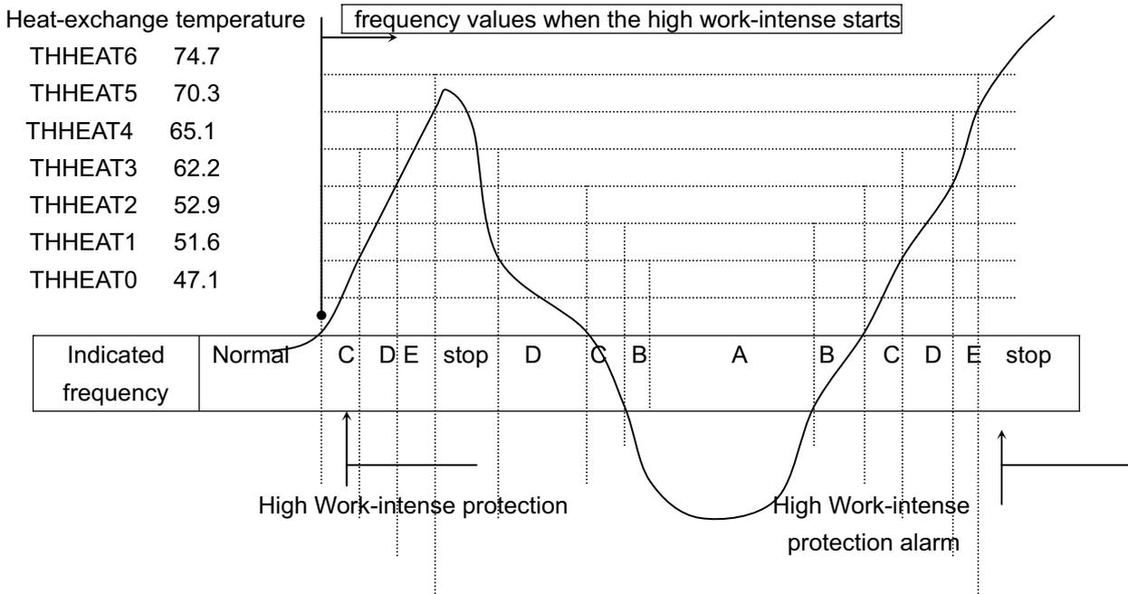
High Work-intense protection alarm will start if there are two times of high work-intense protection within 30 minutes.
