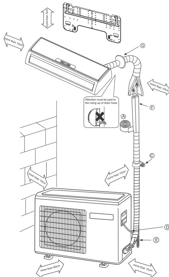
Note: Cooling only units don't have Drain-elbow
