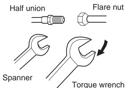
Forced fastening without careful centering may damage the threads and cause a leakage of gas.
