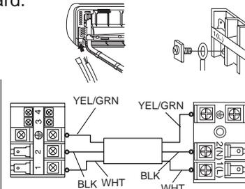
Connecting wiring(with fresh function):  $\geq 3G1.5mm^2+1 \times 0.75mm^2$
