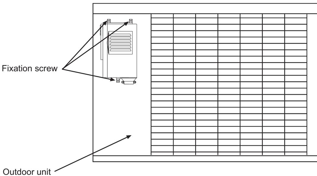
According to the drawing, install the full energy recovery exchanger on the corresponding place of the outdoor unit, and fix the fittings on the outdoor unit cover with the screws.
