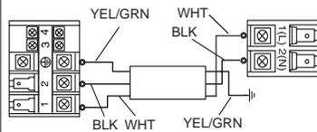
Connecting wiring(with fresh function):  $\geq 3G1.5mm^2+1 \times 0.75mm^2$
