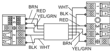
Connecting wiring(with fresh function):  $\geq 5G1.0mm^2+1 \times 0.75mm^2$
