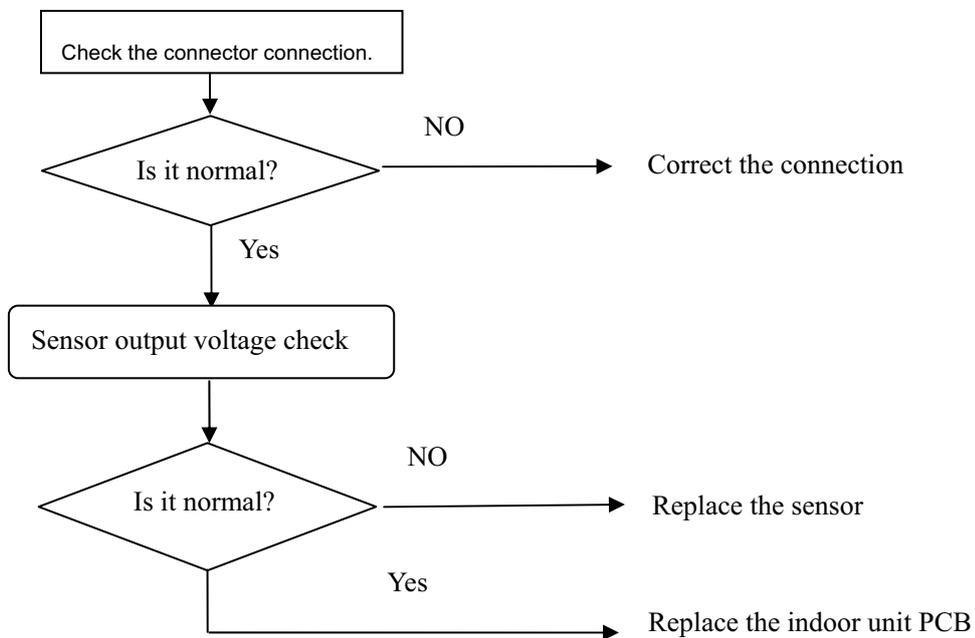
**Sensor output voltage check method:**
