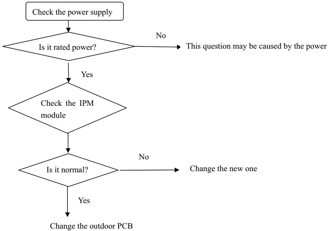
**About how to check the IPM module, please refer to IPM protection fault**
