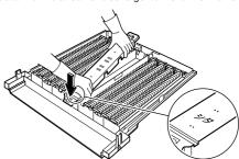
2) Insert top of the streamer discharger.
