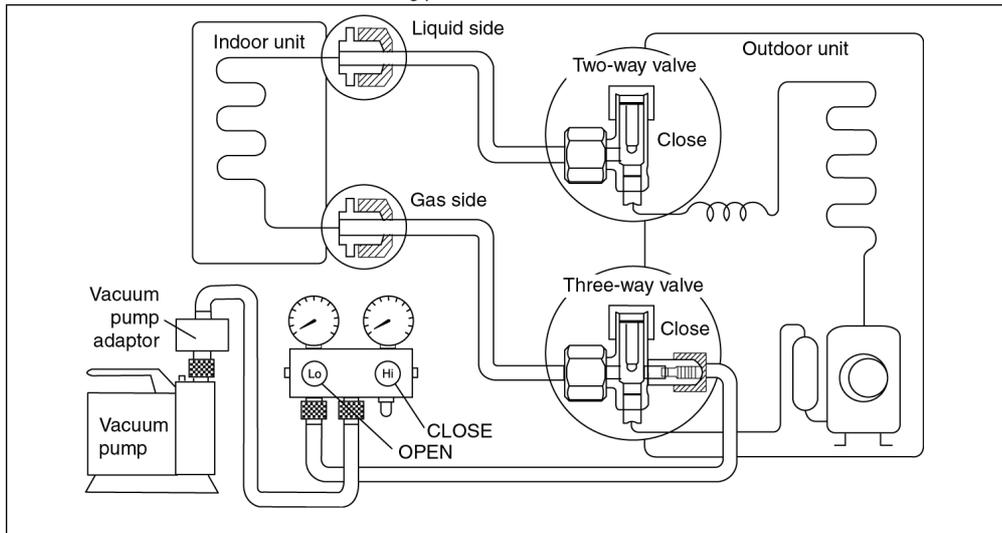
1. Connect a charging hose with a push pin to the Low side of a charging set and the service port of the 3-way valve.
