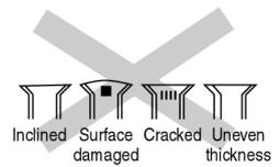
When properly flared, the internal surface of the flare will evenly shine and be of even thickness. Since the flare part comes into contact with the connections, carefully check the flare finish.
