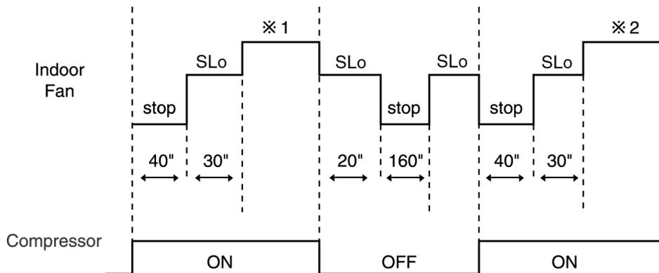
※ 1 Fan Speed is Hi until the compressor stops (when the room temperature reaches setting temperature).
