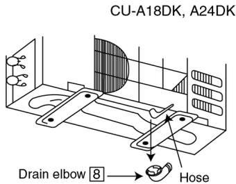
Install the hose at an angle so that the water smoothly flows out.
