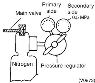
5. Check that the nitrogen is passing through the unit A liquid pipe.
