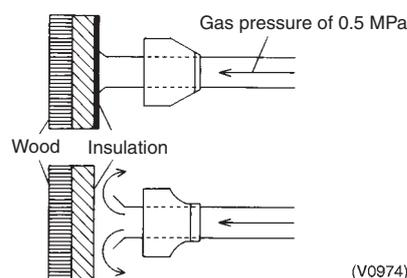
(The nature and amount of the extraneous material inside the pipe can be checked during flushing by placing a rag lightly over the end of the pipe. In the unlikely case that even a small quantity of moisture is found then the inside of the pipe should be dried out thoroughly.)
