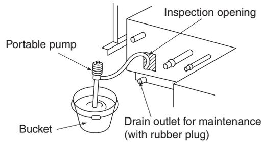
**Note:** Use the drain outlet for maintenance to drain water from the drain pan.
