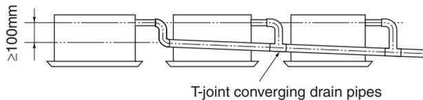
Select converging drain pipes whose gauge is suitable for the operating capacity of the unit.
