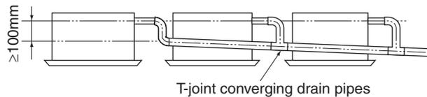
Select converging drain pipes whose gauge is suitable for the operating capacity of the unit.
