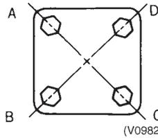
The bolts should be tightened little by little in the above order such that the same degree of torque is applied evenly to each corner.
