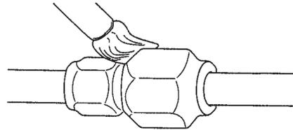
**Tighten the flare but with proper torque.**
