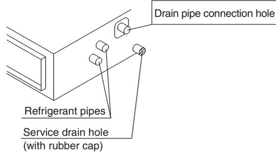
**In case of PVET, NVET (without Drain Pump) Type**
