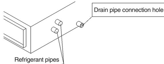
Connect the drain pipe after removing the rubber cap and insulation tubing attached to the connection hole.
