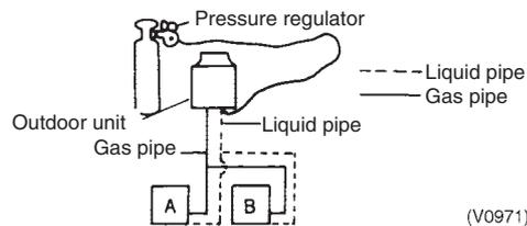
2. Connect the charge hose from the pressure regulator to the service port on the liquid pipe side of the outdoor unit.
