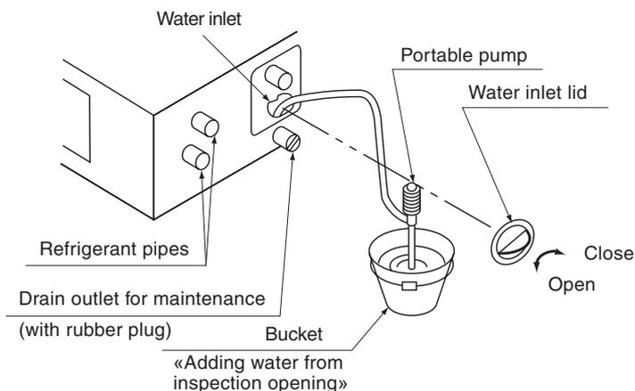
Note: Use this outlet to drain water from the drain pan.
