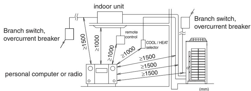
If the electric wave of AM broadcasting is particularly weak, keep distances of 3m or more and use conduit tubes for power and transmission lines.
