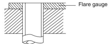
**Size from the dice surface to the copper tip (in mm)**
