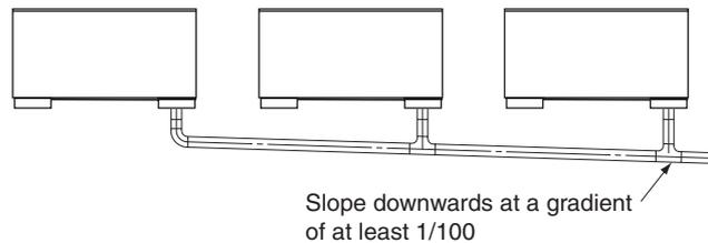
Select converging drain pipes whose gauge is suitable for the operating capacity of the unit.
