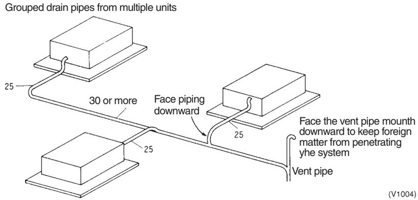
2. The pipework should be kept as short as possible and the number of indoor units per group kept to a minimum.
