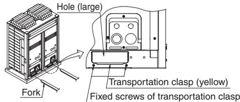
4. If hanging the unit, use a cloth sling to prevent damaging the unit when hanging it. Keeping the following points in mind, hang the unit following the procedure shown in figure 6.
