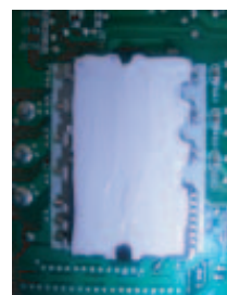
OK : Evenly applied silicon grease.
