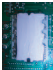
OK : Evenly applied silicon grease.
