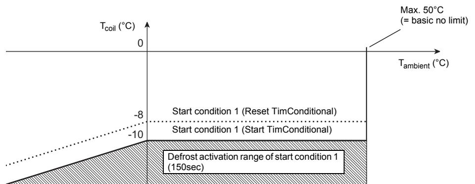
**Start condition 2** The illustration below shows start condition 2 of the defrost function.
