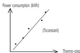
As shown in the left, heat load is calculated from an equation of the first degree which approximates the correlation, among thermo-step, indoor unit's suction air temperature and power consumption, into the linear line under the standard conditions of the unit.
