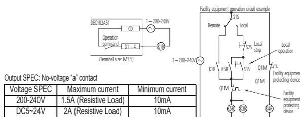
Output SPEC: No-voltage "a" contact
