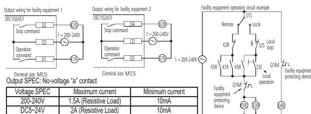
Output SPEC: No-voltage "a" contact
