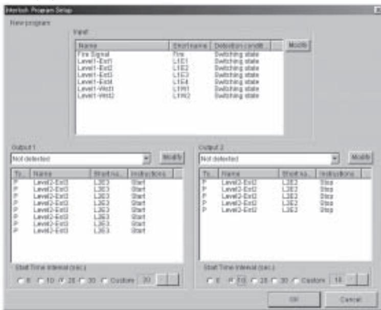
The figure above is an example of a link program that is running air conditioners in common areas along with the air conditioners that are running for certain tenants.
