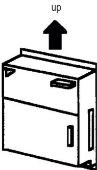
Always attach in the vertical direction. Attaching horizontally will cause failures so do not attach in that direction.
